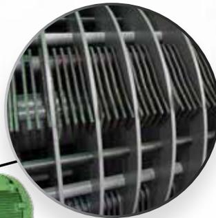
*Grind with hammers optimized for performance and longevity.*
